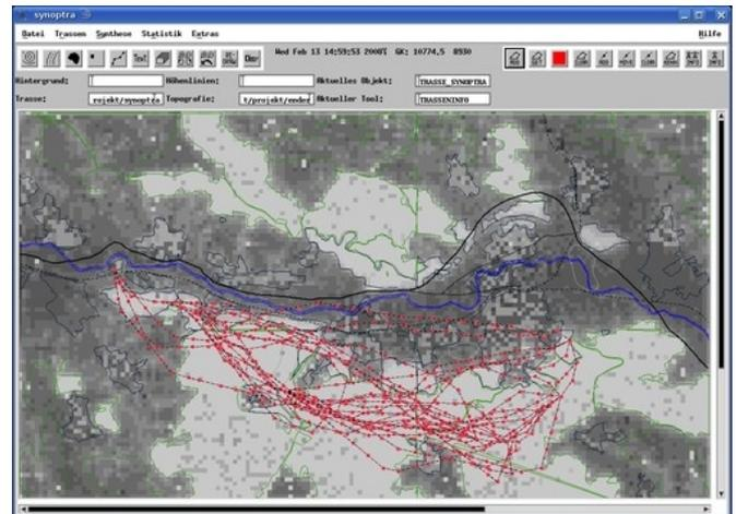
Figure 2: Generation 100 of transmission lines (Visibility optimization)
